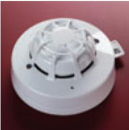
The Discovery UL Multisensor Detector consists of optical smoke and thermistor temperature sensors whose outputs are combined to give the final analog value. As a result, the Multisensor is useful over a wide range of applications and is highly immune to false alarms.
