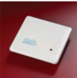
The XP95A Priority Switch Monitor Module is designed to monitor the state of one or more single pole, voltage free contacts and to report the status to Apollo compatible analog control equipment. It can also place a signal on the loop to provide early warning if a device such as a Pull Station is operated.
