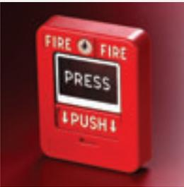
The Addressable Polycarbonate Pull Station is dual-action and features translucent plastic at the center, allowing visibility of an internal LED that indicates alarm condition and polling status. The unit is addressable using a DIP switch protected within the pull station. The Polycarbonate Pull Station may be flush mounted on a single gang work box or use an optional back cover (56000-006).
