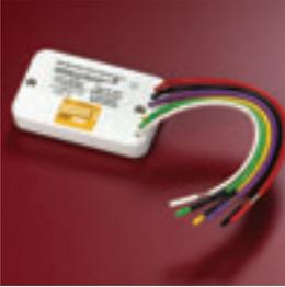
The XP95A Mini Priority Switch Monitor is designed to monitor the state of one or more single pole, voltage free contacts and to report the status to Apollo compatible analog control equipment. It can also place a signal on the loop to provide early warning if a device such as a pull station is operated.
