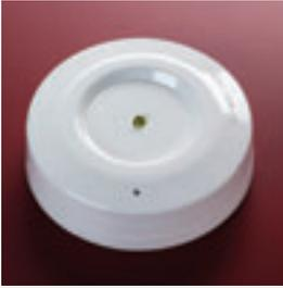
The XP95A Isolator is placed at intervals on the loop and ensures that, in the case of a short circuit, only the section between the isolators will be affected. When the short circuit is removed, the isolators automatically restore power and data to the isolated section.
