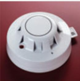
The Discovery UL Ionization Smoke Detector uses a low activity radioactive foil to detect fires by irradiating the air in the smoke chambers and causing a current flow. If smoke enters the chamber, the current flow is reduced leading to an alarm.
