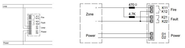
The typical wiring diagram of addressable mode and conventional mode are shown above.
